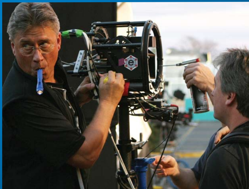
The SI-2K Mini cameras in a stereo rig as used in Dark Country .
